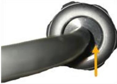
11. Repeat the steps to connect the network cable to the other side of the coupler.
