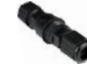
RJ45 IP67 Coupler, p/n 7610203-002. CAT5e/6/6a shielded cable with a 6mm or 8.2 mm O.D. is required for waterproofing
